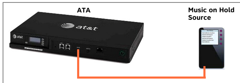
Figure 27. ATA Music on Hold Source Installation
