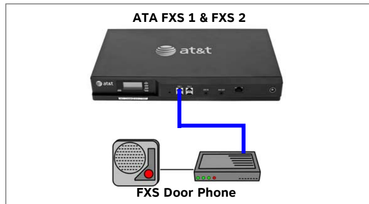
Figure 8. Station Port (FXS) Door Phone Connection
