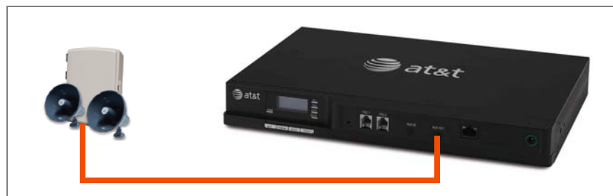
Figure 5. Single-Zone Overhead Paging on AUX OUT Jack
