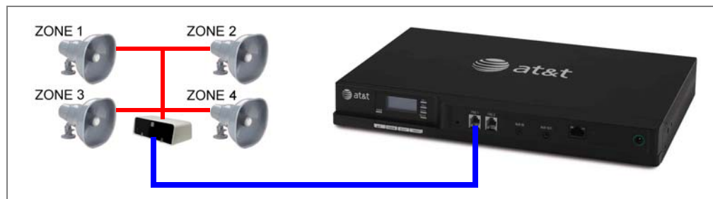
Figure 7. Multiple-Zone Overhead Paging on FXS Port
