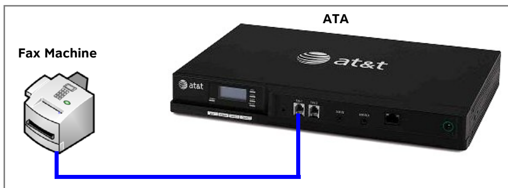
Figure 25. ATA Fax Machine Installation
