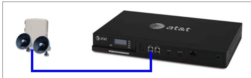
Figure 6. Single-Zone Overhead Paging on FXS Port
