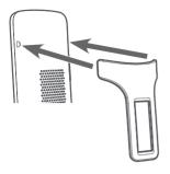
**To attach the belt clip:** Snap the belt clip into the slots on both sides of the cordless handset
