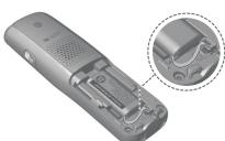
2. Align the cover flat against the battery compartment, then slide it upwards until it clicks into place.
