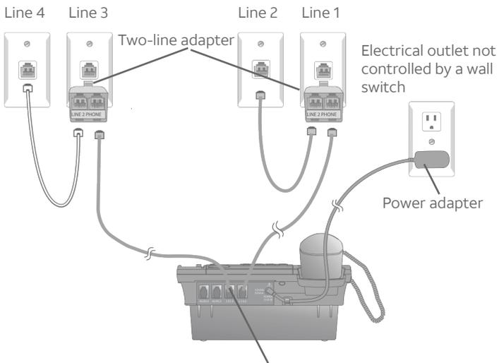
In this installation, four-conductor telephone line cord (RJ 14) is gray. The long cords supplied with the phone are four-conductor cords.
