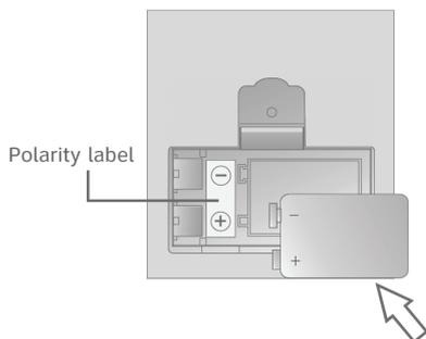
6. Replace the battery compartment cover and tighten the screw. Replace the battery compartment screw with a Phillips screwdriver.
