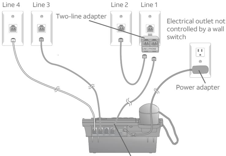
In this installation, four-conductor telephone line cord (RJ 14) is gray.
