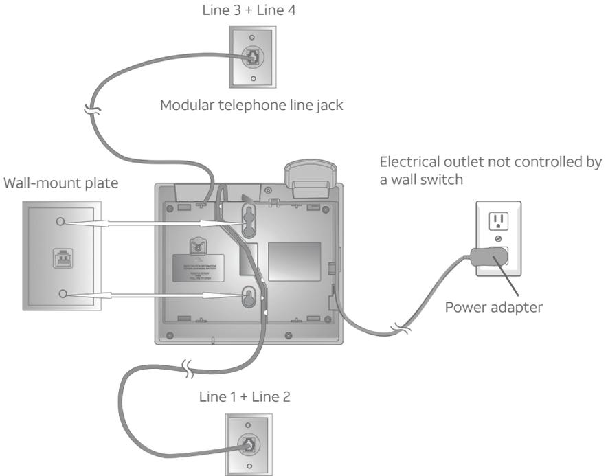
4. Place the telephone base mounting plate (a) just above the mounting studs, then slide the telephone base (b) down until it is secured.
