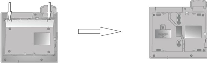
3. Remove the battery compartment screw with a Phillips screwdriver.
