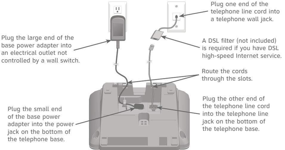
Plug the large end of the charger's power adapter into an electrical outlet not controlled by a wall switch.
