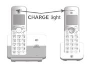
3. Charge the handset by placing it face up in the telephone base or charger. The **CHARGE** light is on when charging.
