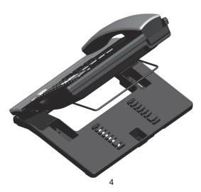
3. Snap the kickstand into the desired grooves until it locks into place.
