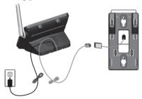
3. Hold the cords to the side of the telephone base. Align the upper slots on the back of the telephone base just above the upper tabs (marked A) of the wall mount bracket. Make sure the lower slots of the telephone base are also aligned above the lower tabs (marked B) of the wall mount bracket. Push the telephone base down until it clicks securely in place.
