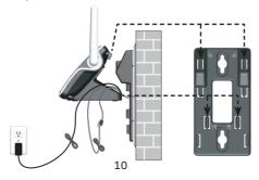
4. Bundle the telephone line cord and power adapter cord neatly with twist ties. Place the bundled cords into the space behind the telephone base.
