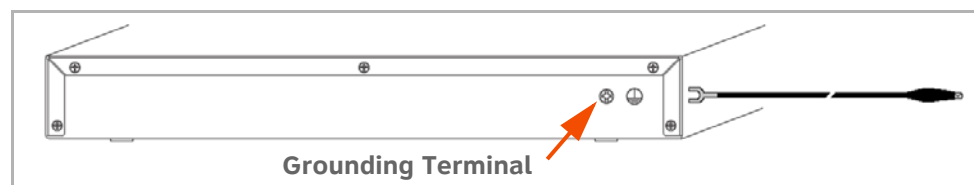
Figure 13. T1 Gateway, SIP Gateway, and ATA Grounding
