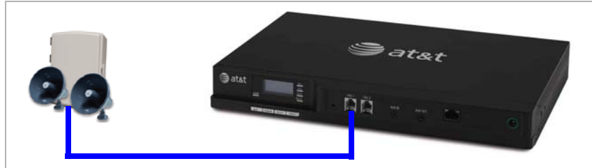
Figure 6. Single-Zone Overhead Paging on FXS Port
