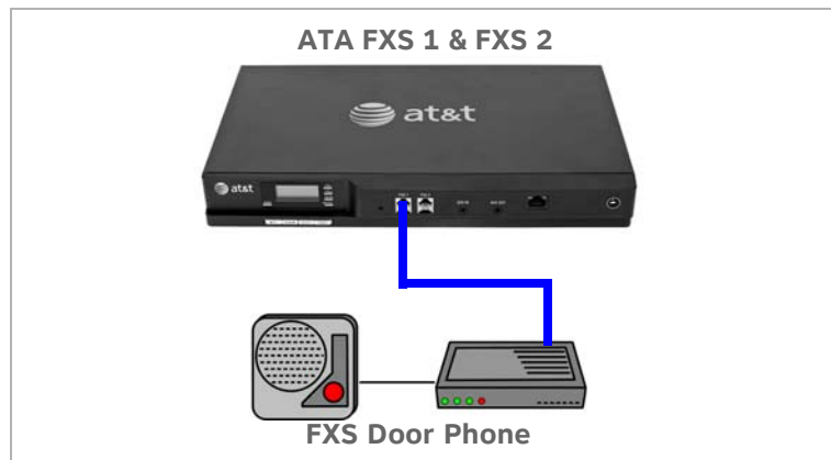
Figure 8. Station Port (FXS) Door Phone Connection
