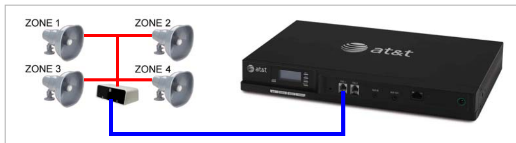
Figure 7. Multiple-Zone Overhead Paging on FXS Port
