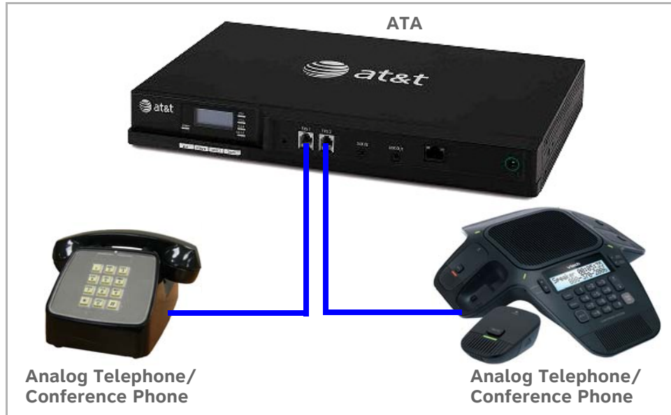
Figure 24. ATA Analog Telephone Connections
