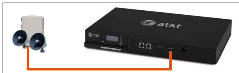
Figure 5. Single-Zone Overhead Paging on AUX OUT Jack
