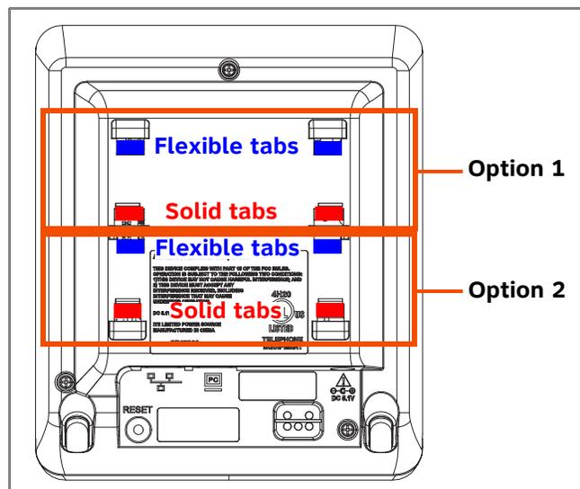
5. Rotate the stand away from you until it rests against the base and you hear a click as the flexible tabs lock into place.
