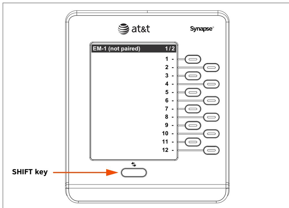
**Figure 6. Expansion Module Front Panel**
