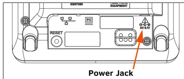
2. Plug the power adapter into an outlet not controlled by a wall switch.
