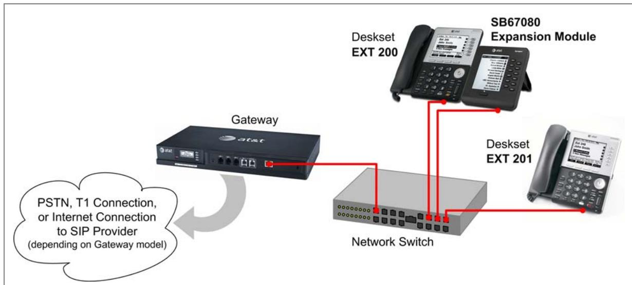
**Figure 1. Expansion Module Network Connection**
