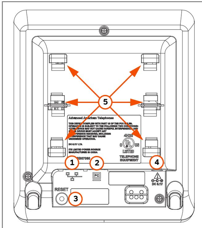
**Figure 3. Expansion Module Connections**
