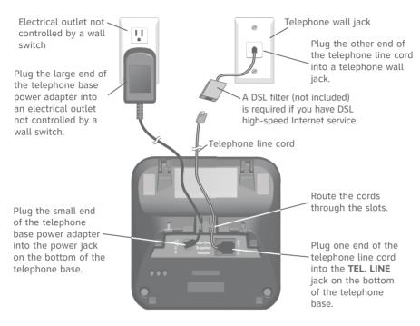
Plug the large end of the charger power adapter into an electrical outlet not controlled by a wall switch.
