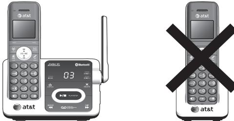
3. The handset displays **Registering handset...** on the handset and the red **IN USE** light on the telephone base turns on. It takes about 90 seconds to complete the registration process. The handset displays **HANDSET X Registered** (X represents the registered handset number). The **IN USE** light turns off and the handset beeps when registration completes.
