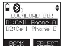
Press **SELECT**. During the download, the handset displays the progress. All other idle system handsets display **Downloading dir**.
