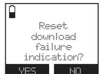
You can also press and hold **OFF/CANCEL** to erase the download fail indicator when the telephone is not in use.
