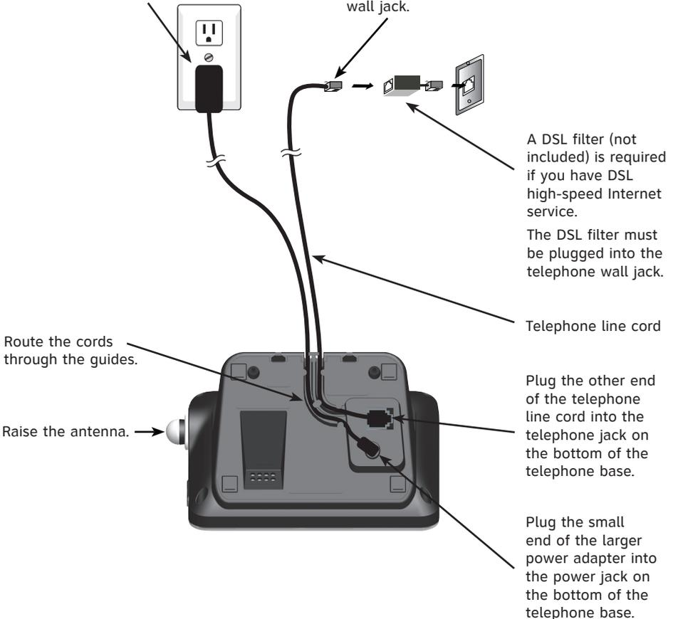
A DSL filter (not included) is required if you have DSL high-speed Internet service. The DSL filter must be plugged into the telephone wall jack.
