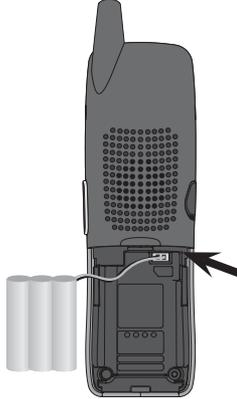
Plug the battery pack connector into handset.
