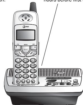
Place handset in base or charger to charge for 16 hours before first use.
