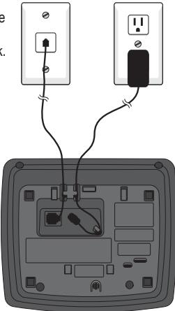
Plug the large power adapter into an electrical outlet not controlled by a wall switch.
