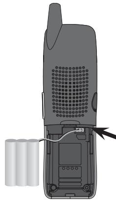
Plug the battery pack connector into handset.
