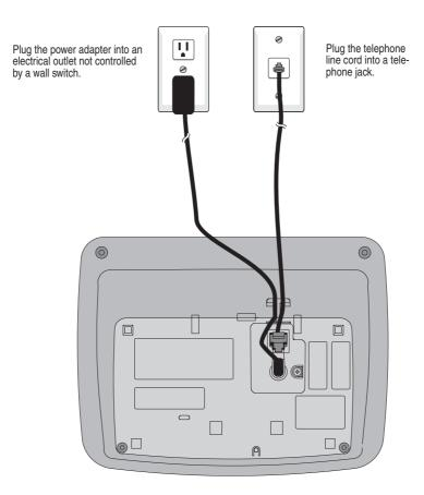
NOTE: Use only the power adapter supplied with this product. If you need a replacement, call 1-800-222-3111. In Canada, call 1-866-288-4268. Be sure to use an electrical outlet not controlled by a wall switch.
