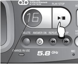
Elapsed recording time (in seconds).
