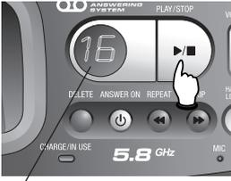
Elapsed recording time (in seconds). Press to stop recording.
