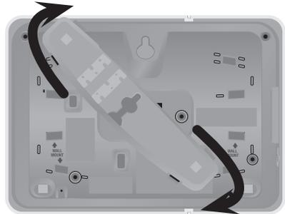
5. Insert the center bracket tabs, then press the bracket downwards until the bracket clicks into place.
