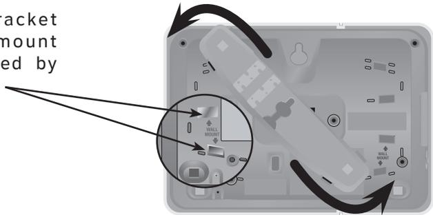
3. Insert the center tabs in first, then press the bracket downwards until the bracket clicks into place and is secured.
