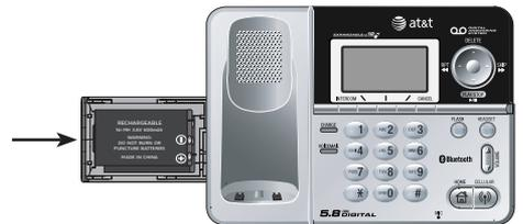
When you have finished installing the spare battery, the battery charging icon will appear in the top right corner of the telephone base display. It takes at least 24 hours for the spare battery to reach a full charge. Once the spare battery is fully charged, you can keep it charged until needed.
