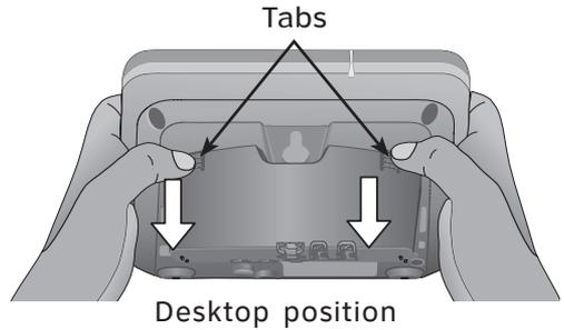
2. Rotate the bracket to the wall mount position indicated by the engravings.
