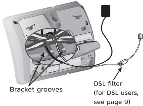
5. Plug the power adapter and telephone line cord into the wall outlets, then align the mounting studs on the telephone outlet plate with the mounting holes on the bracket.
