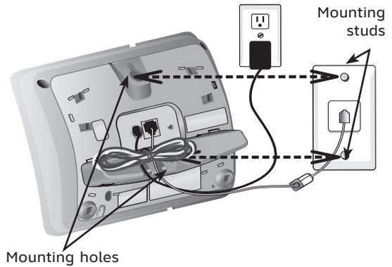
6. Place the telephone base mounting holes just above the mounting studs, then slide the telephone base down until it is secured.
