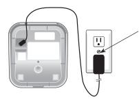
Plug the power adapter into an electrical outlet not connected to a wall switch.
