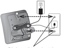
Telephone outlet mounting studs
