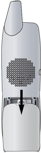
Press tab to open battery compartment.
