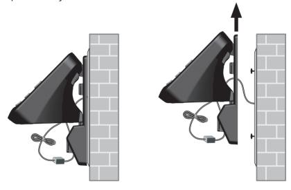
3. Lift the telephone base up to detach it from the wall mount bracket.
