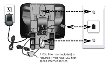
5. Align the holes on the wall mount bracket with the mounting studs of the wall mounting plate and slide the bracket down until it locks securely. Bundle the telephone line cord and power adapter cord neatly with twist ties.
