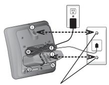
Telephone outlet mounting studs
