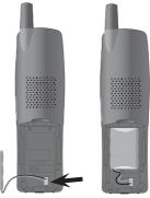
3. Insert the plug as indicated. Be sure to securely insert the plug, making sure that it matches the color-coded label inside the battery compartment.
