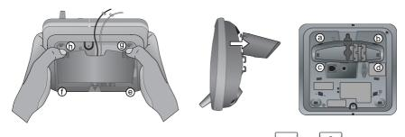
Route cords through slots. Plug the other end of the telephone line cord into a telephone wall jack. Plug the large end of the larger power adapter into an electrical outlet not controlled by a wall switch.
