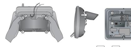
Route cords through slots. Plug the other end of the telephone line cord into a telephone wall jack. Plug the large end of the larger power adapter into an electrical outlet not controlled by a wall switch.
