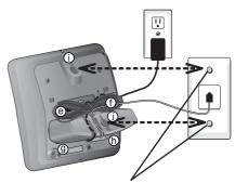
Telephone outlet mounting studs
