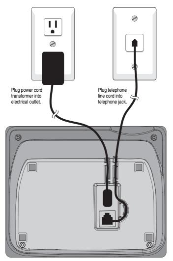
**NOTE:** Use only the power cord supplied with this product. If you need a replacement, call 1-800-222–3111. Be sure to use an electrical outlet not controlled by a wall switch.
