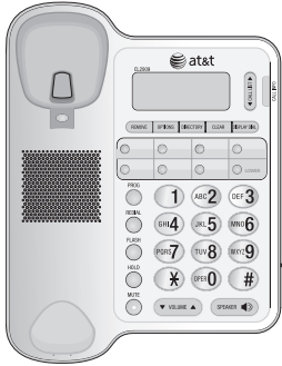
Telephone base with mounting bracket and directory card attached
