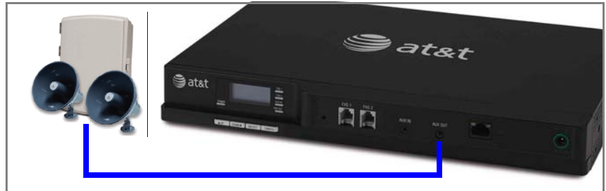
Figure 118. Single-Zone Overhead Paging on AUX OUT Jack
