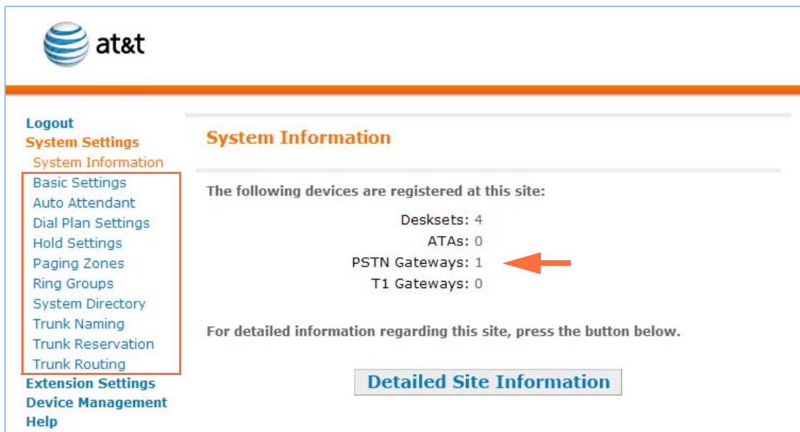
Figure 65. Menu – System Information with a PSTN Gateway and No ATA or T1 Gateway
