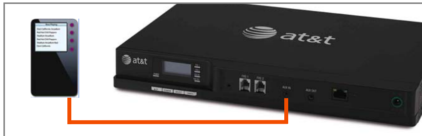
Figure 114. Music on Hold Source Connected to the AUX IN Jack
