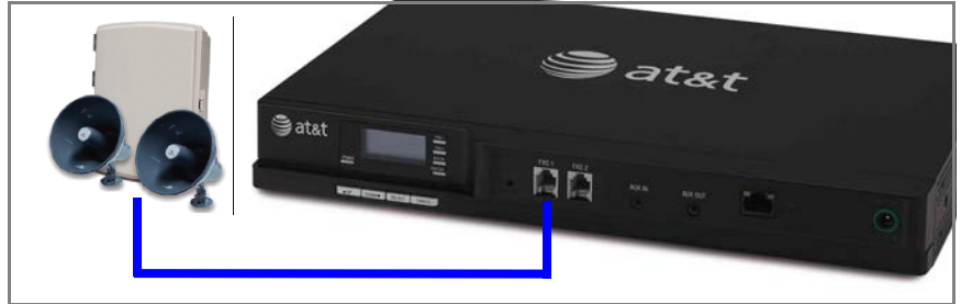
Figure 119. Single-Zone Overhead Paging on FXS Port
