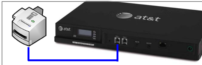
Figure 105. Fax Machine Connected to FXS Port
