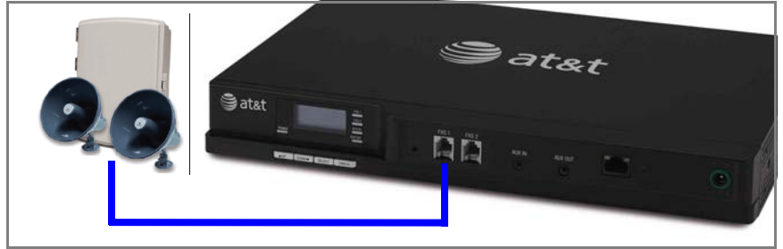
Figure 101. Single-Zone Overhead Paging on FXS Port
