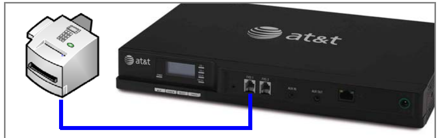
Figure 87. Fax Machine Connected to FXS Port
