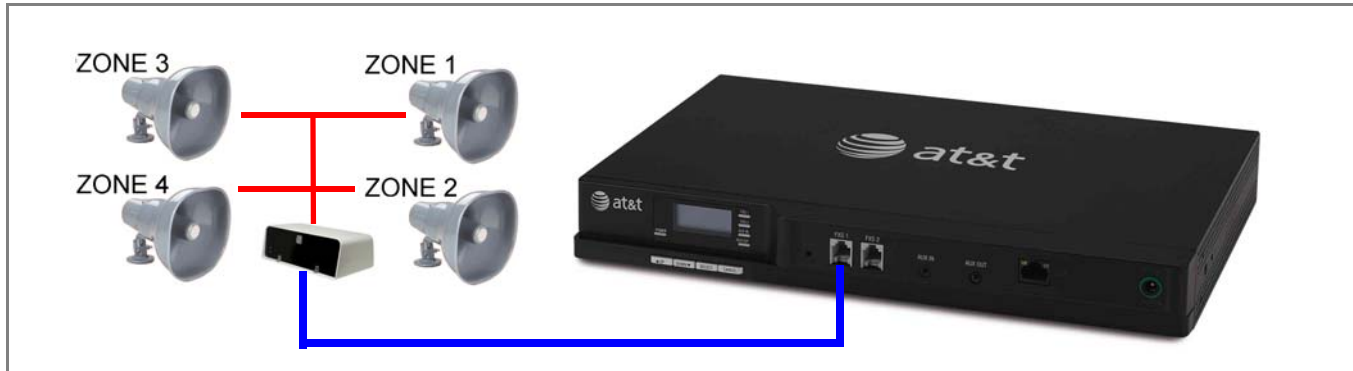
Figure 102. Multiple-Zone Overhead Paging on FXS Port
